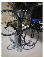
Whether it's changing a flat or adjusting brakes and derailleurs, the bike repair stand features an air pump, tools and mounts so riders can securely hang a bike and make adjustments. The repair station is one of 16 stands to be installed by the County. Additional units will be located in high traffic biking communities near fire stations.
