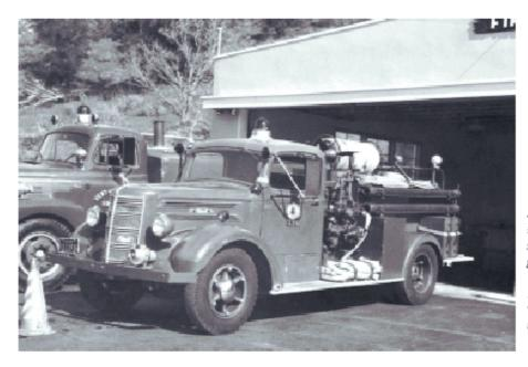
Fire Station 33 first engine #276, 1942 Mack, 500 gpm skid mount pump and 400 gal. Water tank.
