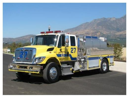
The water tender is a large tank truck used to carry water to fire engines when a water source is not readily available. Typically, this is in remote or rural areas where fire hydrants are not available. Water tenders are often deployed during brush fires, but a water tender can also be relocated to an urban area, if the hydrant system is not working.
