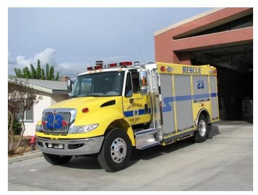
The Rescue unit carries the specialized tools and equipment needed to support firefighting operations and rescues. A rescue unit responding with an engine forms a rescue engine (see Rescue Engine). There is also a smaller Rescue unit in the department.
