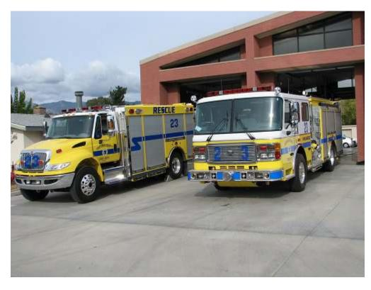
A rescue engine is an engine combined with a rescue unit forming a two-piece company. It has the capabilities of an engine, plus with the specialized equipment carried on the rescue, it can perform the functions of a truck. It lacks only the aerial ladder and complement of ground ladders carried on trucks.
