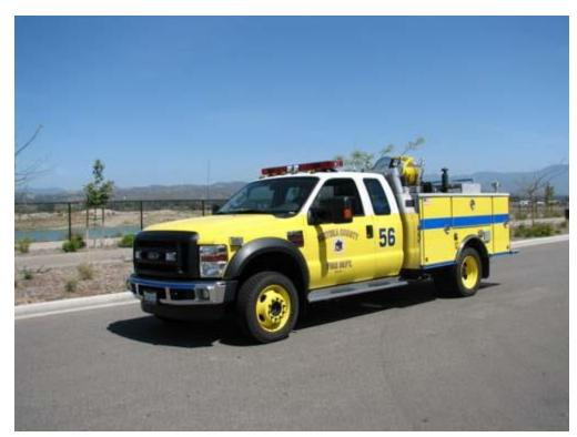
A patrol is a 4 wheel drive heavyduty pick-up truck with a slide-in pump unit. The pump unit has a small diesel engine driving a pump, a 280-gallon water tank and small diameter hose on a reel for rapid deployment. It is designed to do a quick attack on a small brush fire.
