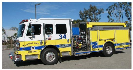
A medic engine performs all the functions of a standard first-run engine, but is also capable of ALS (advanced life support) service. The firefighter assigned to a medic engine is a paramedic, trained and certified to perform ALS. The engine carries, in addition to the normal inventory of equipment, the specialized equipment and medical supplies the paramedic needs.
