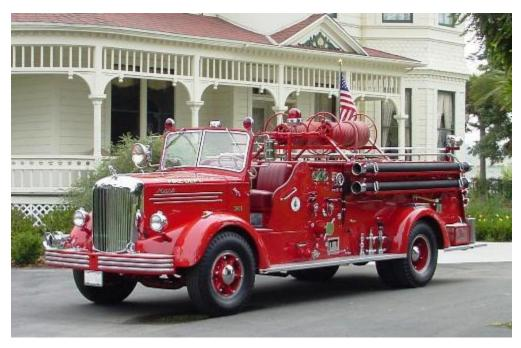
The Mack parade engine is a 1948 Mack 750-gpm (gallons per minute) pumper. It was originally put into service with the Ventura County Fire Department in 1948, and served for 40 years as a firstrun or reserve engine until it was retired in 1988. It was purchased at auction by a Fire Captain and then donated back to the department.
