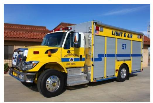
The light and air unit supports emergency operations. A special air compressor system refills the air cylinders for the SCBA (self-contained breathing apparatus) used by firefighters in a fire. The unit also carries a supply of spare air cylinders.
