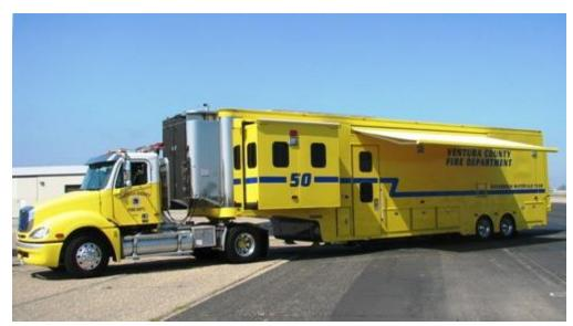
The hazmat (hazardous materials) unit responds on incidents involving hazardous chemical, radiological, biological, explosive or unknown materials. At the front of the trailer is a workstation with reference materials and computers that can be used to identify materials and command the hazmat aspect of operations while on the scene of an emergency.
