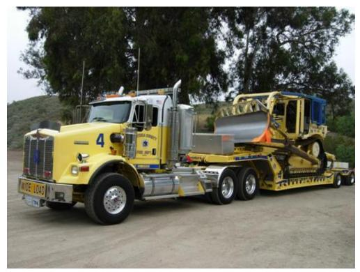
Within the VCFD, bulldozers are referred to as "dozers." The dozer is a three-piece unit consisting of the dozer, the tractor/trailer used to transport it and dozer-tender truck. Dozers have an enclosed, air-conditioned and protected cab for the safety of the operator.
