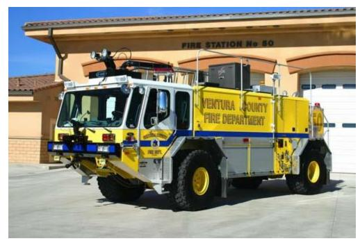
The crash/rescue truck is a specialized unit designed to fight large flammable liquid fires, in particular aircraft fires. It can also be utilized on gasoline fires in refinery or storage settings, or a tanker truck on the highway.
