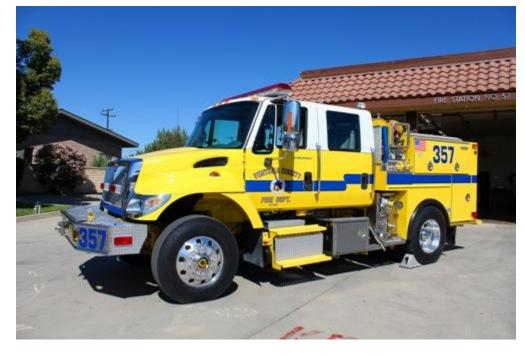
A brush engine is smaller than an urban/structural engine. They are designed for rural/wildland firefighting where access is limited and roadways are not always available. The equipment and components are oriented toward fighting brush fires.
